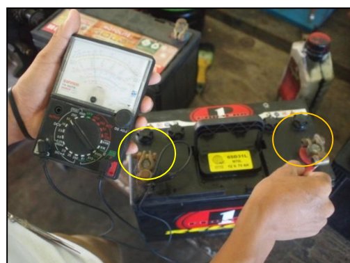
Connection of tester when testing voltage
