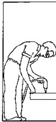
SOLDERING IRON WITH BENT HANDLE ALLOWS ELBOW TO BE LOWERED AND WRIST STRAIGHTENED GOOD DESIGN
