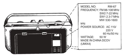
In this example, the power rating or wattage of the radio is 50 watts or 50 W. Look at the back of some of the appliances in your house. Try and identify the power rating or wattage and record it in the table below.
