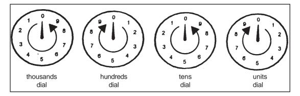
All the pointers rotate when electric power is being consumed. The units pointer rotates the fastest while the thousands pointer rotates the slowest.
