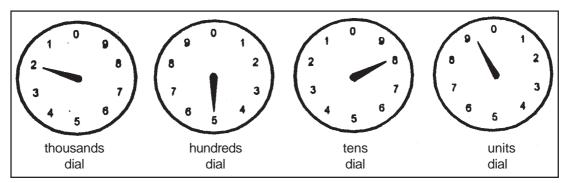
The pointer of the units dial and the hundreds dial rotate clockwise while the pointer of the tens dial and the thousands dial rotate counter-clockwise.
