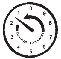
Observe the four dials in the electric meter carefully. There are ten numbers on each dial: 0, 1, 2, 3, 4, 5, 6, 7, 8 and 9. The numbers in each dial are read in sequence from left to right. The first dial indicates the thousands dial, the second dial is the hundreds dial, the third is the tens dial and the fourth is the units dial.
