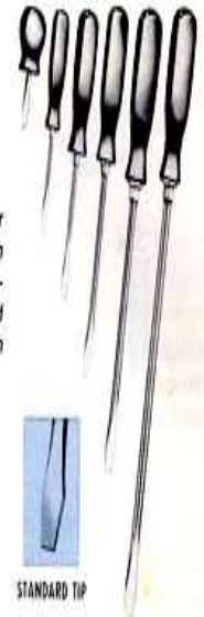
Fig. 4-38. The body repair worker needs a good selection of standard (straight) tip screwdrivers. These have a round shank. (Courtesy of Snap-On Tools)
