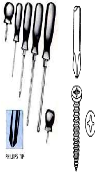
Fig. 4-40. Phillips® screwdrivers are a necessary part of the body worker's tool kit. Phillips-head screws are often used to fasten interior trim parts. (Courtesy of Snap-On Tools)
