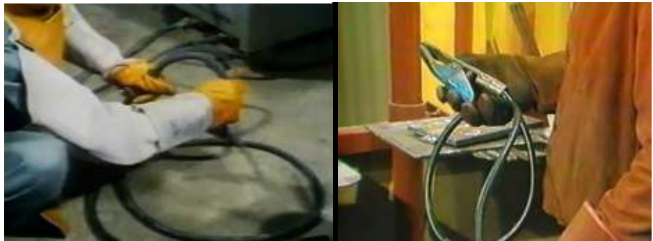
Check welding cable for crack or cut insulation
