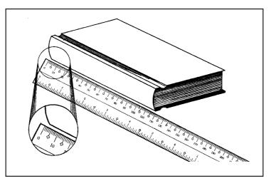
With the zero mark fixed on one end of the object, measure the length by reading where the gradations on the ruler meet the other end of the object.
