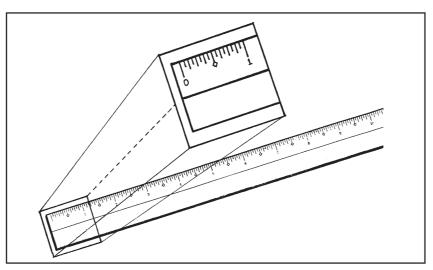
Notice that there are 16 gradations in one inch. Each gradation is  $1/16^{th}$  of an inch. The gradations of an inch are:
