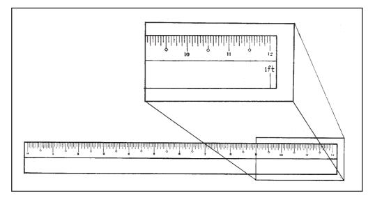
When an object cannot be measured in whole foot units, the measurements are expressed in feet and inches; i.e. 5 feet and 6 inches, 4 feet and 11 inches, etc. This is usually how people measure their height.
