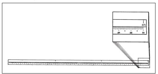
The yard is usually used for measuring objects of great length like rolls of cloth, sheets of aluminum or coils of wire. It may also be used to measure short distances.
