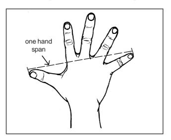
To measure the length of an object using the hand span, place your outstretched hand at one end of the object. Then move your hand along the object, always beginning the next hand span at the point reached by your little finger. Count how many hand spans you are able to make from one end of the object to the other. Record your results.
