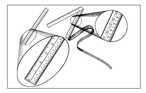
Observe the gradations of the ruler in centimeters and that in millimeters. Do you notice the similarity? For gradations expressed in centimeters, the count is 1, 2, 3, 4, 5 and so on. For gradations expressed in millimeters, the count is 10, 20, 30, 40, 50 and so on. These marked gradations are actually equal in length. This means that 1 cm = 10 mm, 2 cm = 20 mm, and so on.
